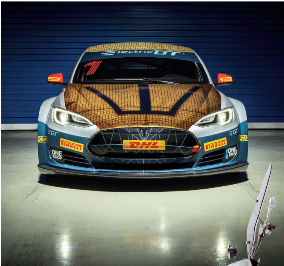
FIG. 19 Car roof top and hood made from a twill 2/2 flax fiber weave and a reinforcing grid. (ampliTex and powerRibs – BComp – Electric GT)
