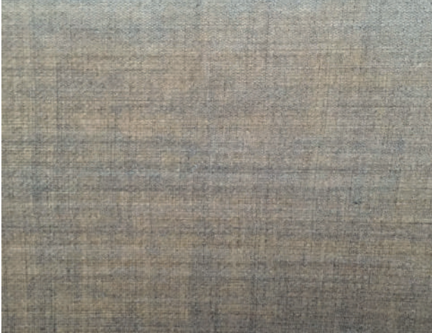
FIG. 17 Thermoplastic woven flax fiber prepreg with 40wt% PP.
