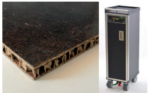
FIG. 31 Flax fiber random mat/furan fire-retardant sandwich, used as side panels in a lightweight trolley for aircrafts, reducing fuel consumption. (Fibrirock sandwich, Ecotechnilin, used in SmartCart)
