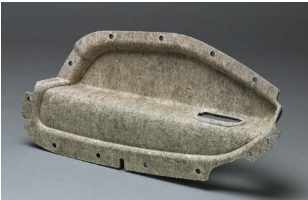
FIG. 15 Overmolded car door panel containing flax fiber/PP random mat on the inside and pure PP on the outside to form the intricate details. (FibriPlast Hybrid by Ecotechnilín used by Mercedes - E class)
