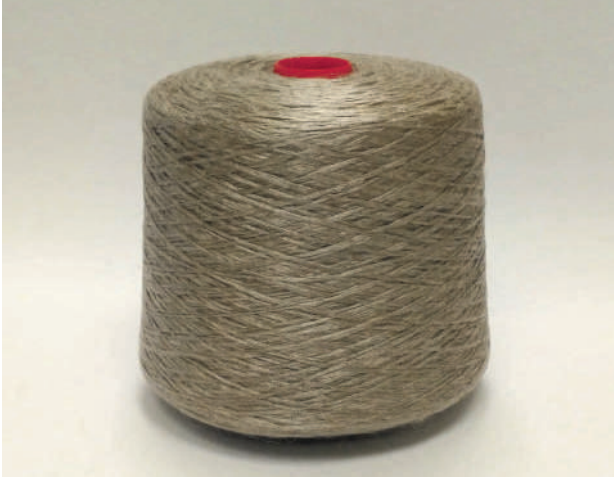
FIG. 5 Flax fiber roving with a linear density of 400 tex.
