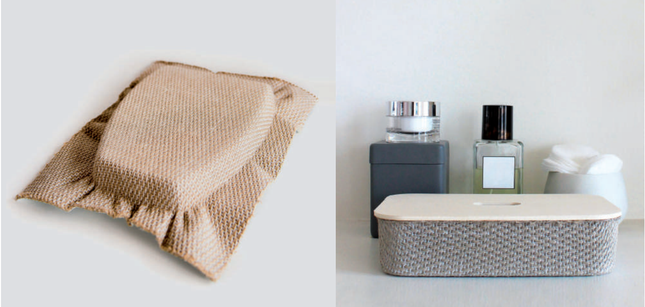
FIG. 17 A box made from a flax fiber/PLA woven prepeg. The weave contains PLA filaments that can be melted to impregnate the flax fibers. In this application, the filaments were only partially melted to give the box a more natural aspect. (Varian by CultureIN used in Designerbox 36 by Philippe Nigro)
