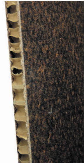
FIG. 15 (Left) Non-woven flax fiber mat pre-impregnated with PP. The mat consists of 50 wt% flax fibers and 50 wt% PP filaments, which are intimately mixed during production. (Right) Consolidated non-woven furan prepreg containing 30 wt% flax fibers used as skins in a sandwich panel.
