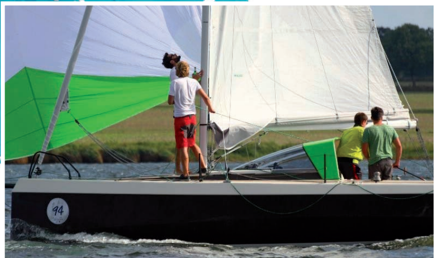
FIG. 24 Leisure boat comprising several deck parts made of woven flax fiber epoxy composites. (ampliTex - BComp used by Greenboats)
