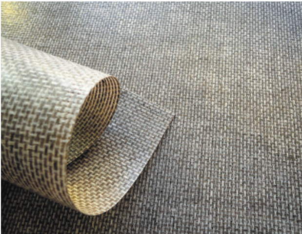
FIG. 18 Woven flax fiber prepreg with polyamide 11 resin.
