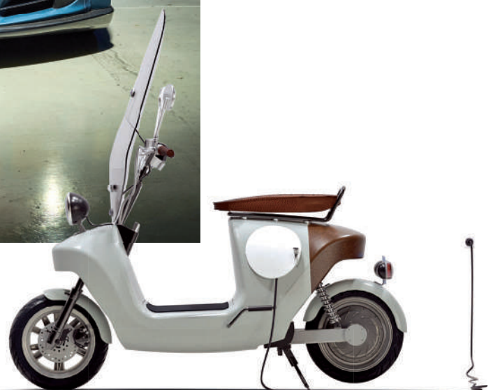
FIG. 20 Scooter with a flax- and hemp-fiber random mat reinforced body. (Flax fibers - Van de Bilt Zaden en Vlas used in Be.e scooter – Van.Eko)
