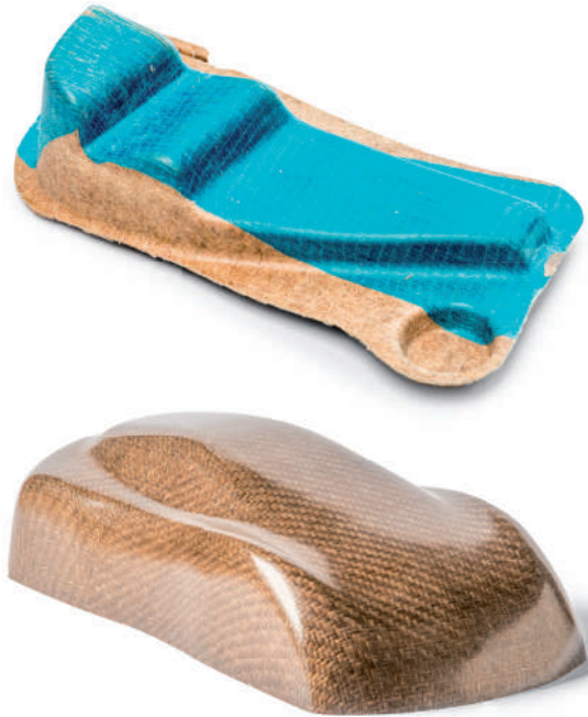
FIG. 35 Decorative designs based on flax & hemp fiber composites are becoming increasingly popular in the automotive industry. In addition, in-mold decorations can produce even more visually appealing parts. (BComp)
