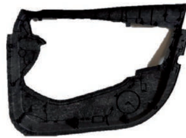
FIG. 15 Overmolded car door panel containing flax fiber/PP random mat on the inside and pure PP on the outside to form the intricate details. (FibriPlast Hybrid by Ecotechnilín used by Mercedes - E class)
