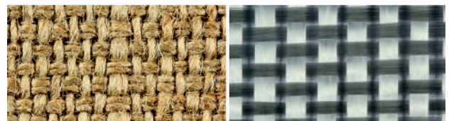
FIG. 3 Balanced woven fabric of fibers, orientations 0° and 90°, (a) flax, (b) glass
