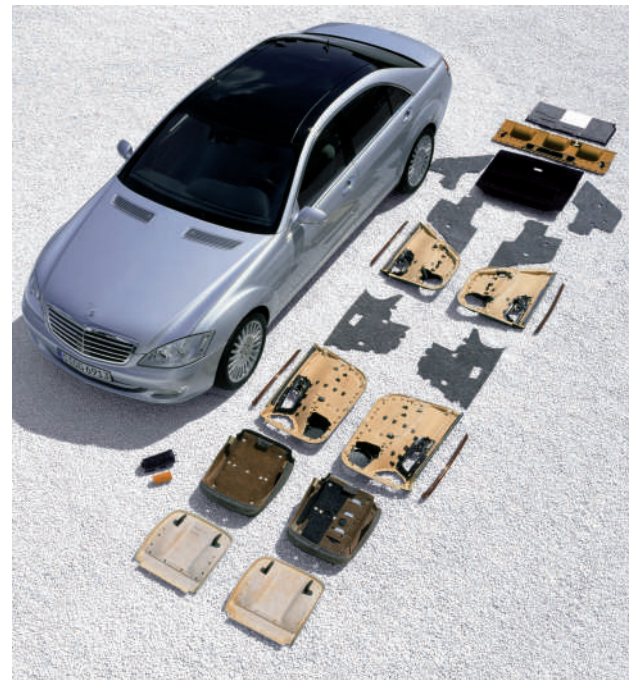
FIG.11 The approximately 45kg of natural fibers in a Mercedes S-Class. (Source: Daimler)
