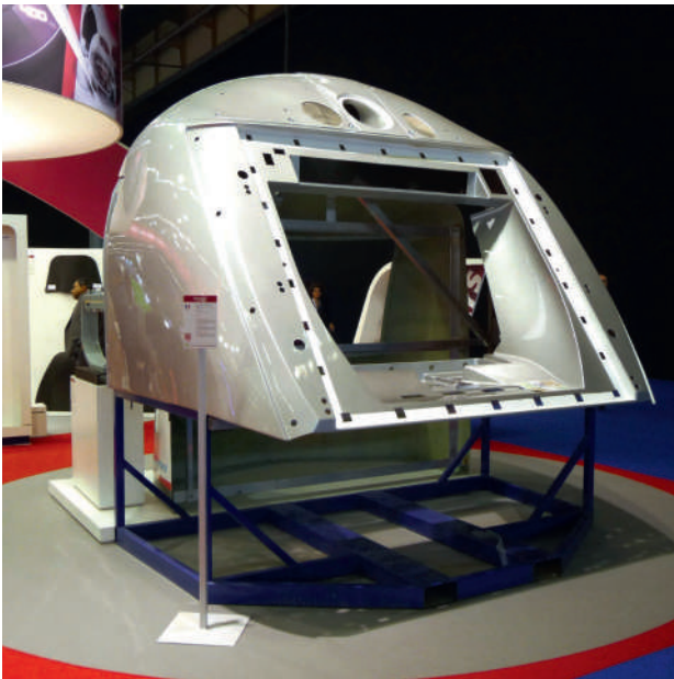
FIG. 32 Train cabin containing 37.5 wt% of woven and non-woven reinforcements in a polyester resin. (F.R.D.)
