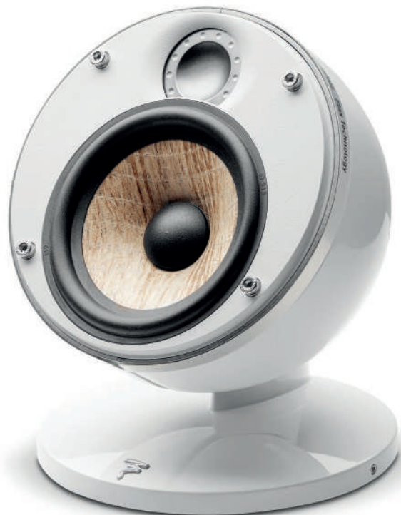
FIG. 18 Speaker diaphragm consisting of a quasi-UD flax fiber/PP weave in between two glass fiber sheets. (Quasi-UD weave Biorenforts by Terre de Lin used by Focal)
