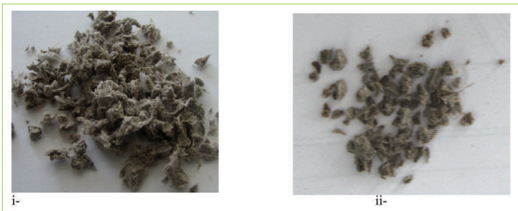
Figure 8: Effect of the processing parameters on the quality of granulates after mechanical cutting: i- fluffy, unsuitable for injection moulding process; ii- properly cohesive granulates with pourable properties for injection moulding.
