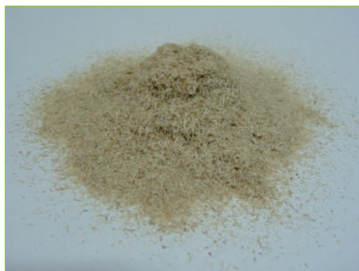
Figure 4: Very short crushed fibres, which are powder-like. (Source: FRD)
