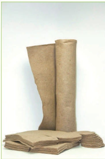
Figure 5: Non-woven flax mat produced by needlepunching. (Source: ECOTECHNILIN)
