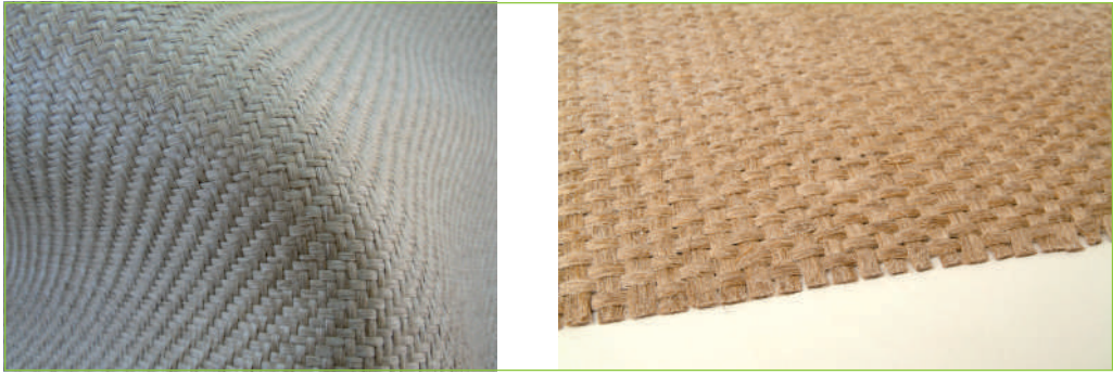
Figure 12: Commingled weave of flax with thermoplastic matrix (left) - (Source: Groupe Depestele); Thermoplastic prepreg of flax weave with powder (right) - (Source: Dehondt Groupe).
